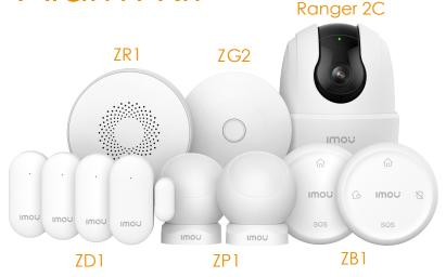
The Alarm Kit includes: ZG2 gateway, ZB1 remote control, ZD1 door and window sensor, ZP1 motion sensor, ZR1 Alarm Siren, Ranger 2C Camera. The products of the Alarm Kit can be linked with the IMOU camera through the APP scene setting. You can also activate or disable the entire security system at will.
